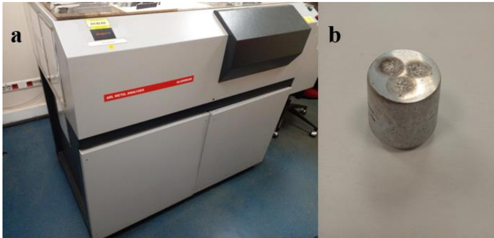
Figure 2.9: a) Thermo-scientific Thermo ARL3460 Metal Analyser Device and b) OES specimen example of DoE set.
