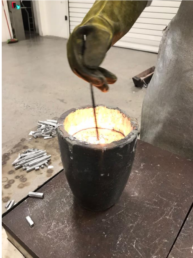
Figure 2.3: Master alloy inoculation with manual stirring process for A356 melt.
