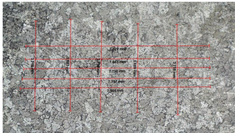
Figure 3.17: Grain size measurement example.
