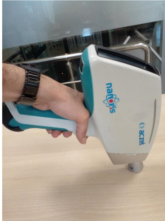
Figure 2.10: Aczet Portable XRF Device measurement visualization.
