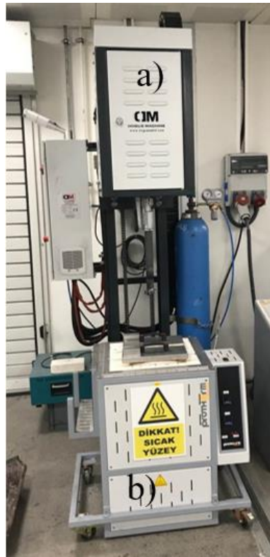
Figure 2.4: a) Rotary Degassing Machine and b) continuous heating furnace that designed to work as pair.
